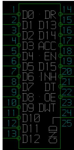
Figure 3.2.1. – D-25 connector pinout
